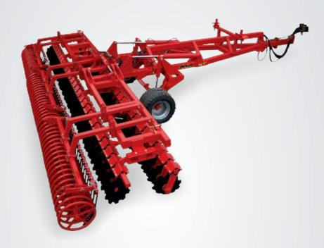
For many years, short disc harrows manufactured by KNOCHE are a decisive factor in the area of passive soil tillage.
