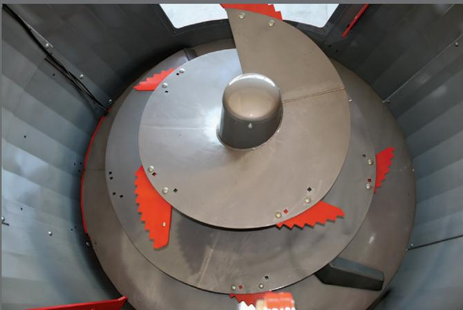
All the auger parts (coils and cones) are made of K-NOX to protect the entire unit. The auger is more resistant to abrasive fodder and acidic silage juices.
