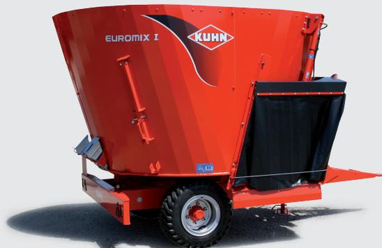
The single auger EUROMIX I comes in 8, 10 and 12 m<sup>3</sup> versions with a vertical auger, providing mixed rations for all types of livestock farms. The shape of the tub and the auger design were specially engineered to ensure optimum circulation of the forage products in the machine and guarantee an even mix. The counter-knives are articulated at the top to provide a large chopping surface.
